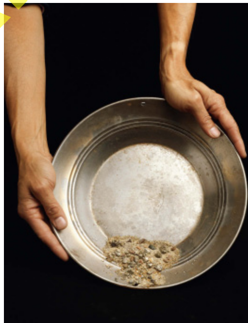
Figure 6.39 Gold panning is one of the oldest and simplest ways of extracting gold.
