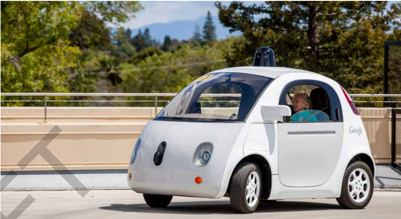
Source 3 Google has successfully designed a self-driving car. The cars use their sensors and software to detect objects such as pedestrians, cyclists and vehicles, and are designed to safely drive around them.
