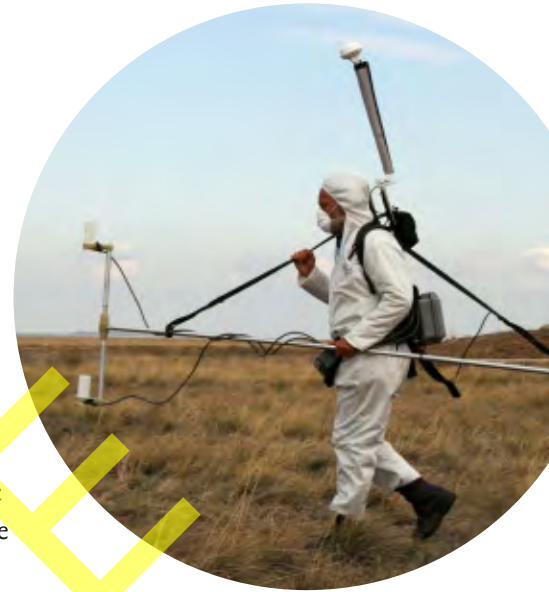
Figure 5.38 A magnetometer is used to measure changes in the Earth's magnetic field.
