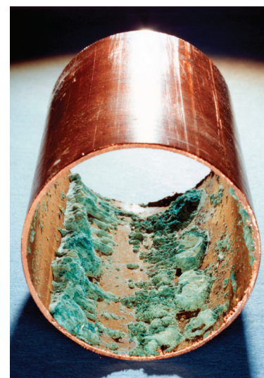
Figure 3.22 All metals corrode, but only iron forms rust. The corrosion of this copper pipe produced copper oxide, which then reacted further with carbon dioxide to form green copper carbonate.
