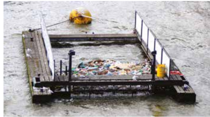
Source 4 Modern cleaning of the Thames; this device collects floating rubbish, such as plastic and wood.
