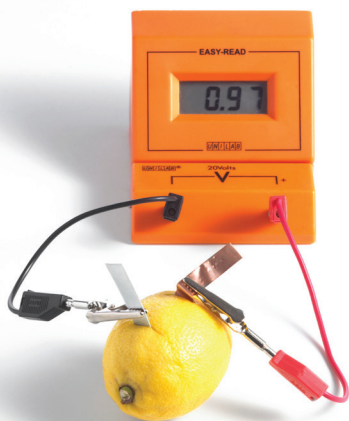
Figure 4.14 Adding appropriate electrodes and connecting wires to a lemon can produce an electrical current.
