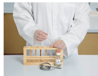
Figure 4.6 (a) Add dilute HCl to a magnesium strip and (b) quickly invert a second test tube over the first to catch the hydrogen gas formed.
