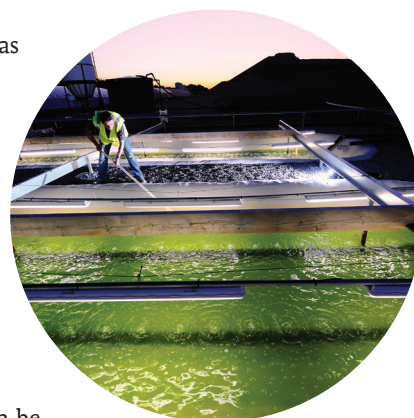
Figure 4.57 Microalgae are now being farmed to metabolise household wastes and produce methane as a fuel. The carbon dioxide produced in burning the fuel is then pumped back into the tanks to help promote photosynthesis.
