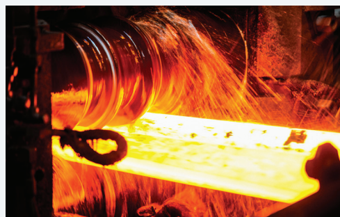
Figure 4.38 Hot iron being roll-pressed into a length of rail.
