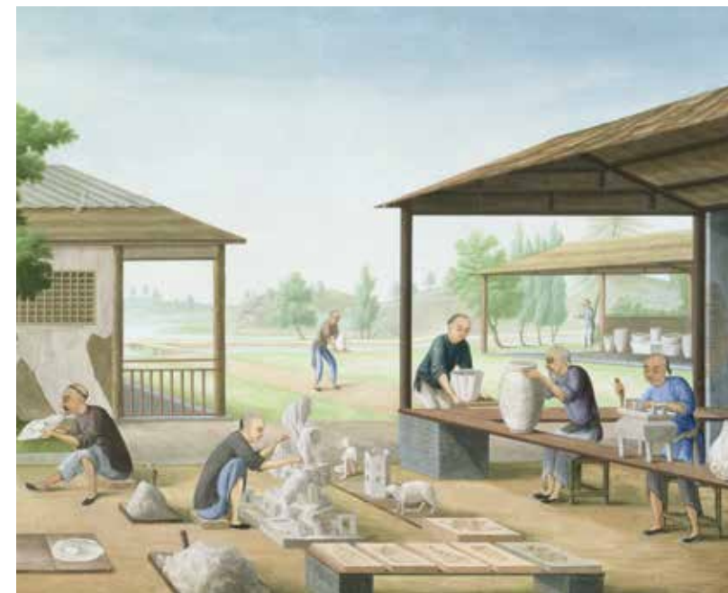
Source 3 A painting from the 19th century depicting the manufacturing of porcelain in China using hand modelling and moulding techniques
