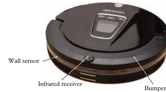
Figure 4 Robot vacuum cleaners send infrared beams around a room to tell the robot the size of the room and if there are any drop offs like stairs.
