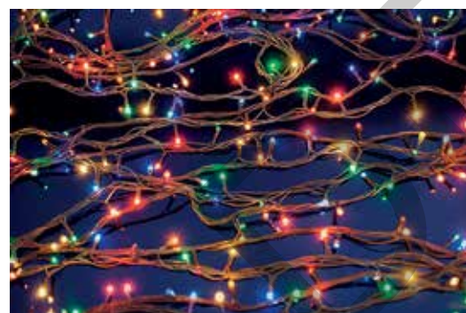
Figure 2 Traditionally, party lights were a series circuit. This meant that when one light broke, all the lights went out. Now, most modern party lights are arranged in a parallel circuit.
