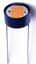
Figure 6.48 Many types of resistor are available. (a) The resistance of carbon resistors is indicated by the coloured bands on their plastic case. (b) The resistance of a light-dependent resistor (LDR) varies depending on the brightness of the light shining on it. This makes LDRs useful in sunset sensors that control automatic lighting circuits, like street lights or security lights.
