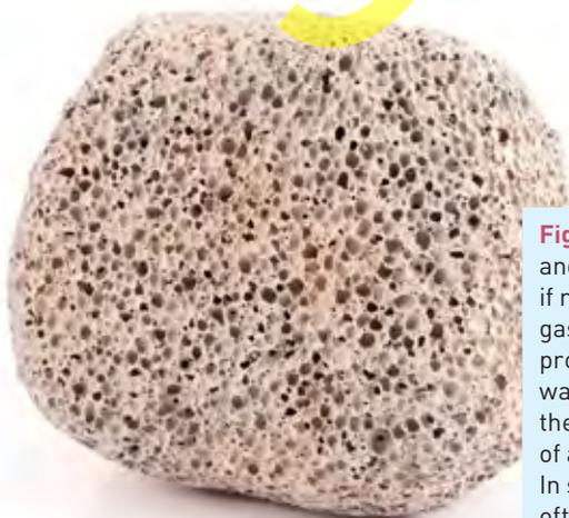
**Figure 2.1 Weight** and density are less if rocks contain large gas holes that were produced when the rock was formed. In pumice, the holes can be the size of a match tip or smaller. In scoria, the holes are often the size of a pea.
