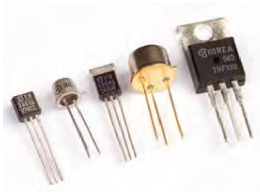
Figure 3.42 Transistors come in different shapes and sizes. The miniaturisation of transistors has revolutionised electronics and computing.
