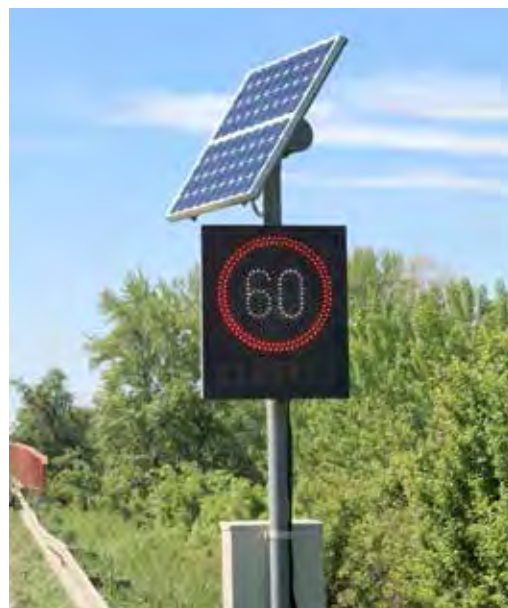
Figure 3.46 Solar-powered signs are becoming common all across our country. These signs transform solar radiation into light energy.
