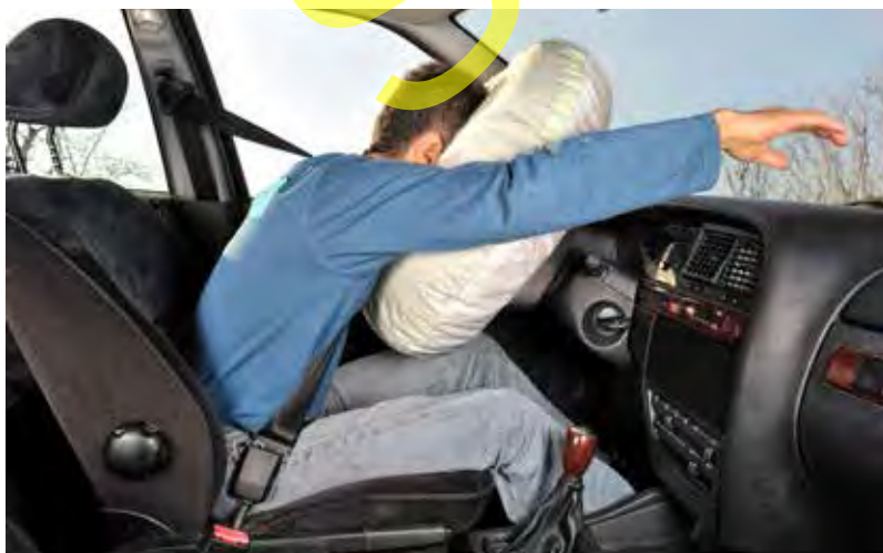
Figure 3.10 Seatbelts and airbags in cars are designed to slow you down before you stop in a crash, reducing the kinetic energy and hopefully preventing injury.
