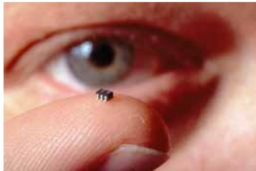
Figure 3.43 When it was introduced in March 1998, this operational amplifier, containing 50 transistors, was the world's smallest integrated circuit. Even smaller integrated circuits are now used in phones, games and many other electronic devices.
