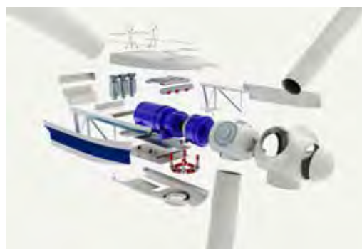
Figure 3.55 The generator inside a wind turbine.
