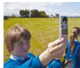
Source 3 This boy is measuring wind speed with a hand-held anemometer
