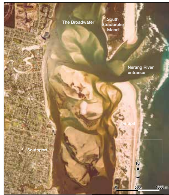
Source 1 Aerial photograph of the Nerang River entrance, 1984. You can see how the southern tip of South Stradbroke Island has been eroded by the waters flowing out of the river.
