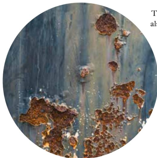
FIGURE 8 The corrosion of iron metal forms rust, seen here as red-brown patches.
