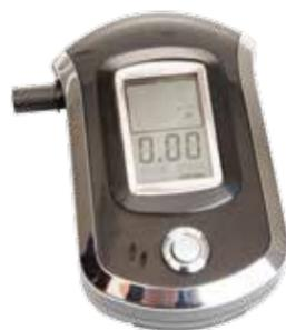
FIGURE 2 A breathalyser can be used to estimate BAC from a breath sample.
