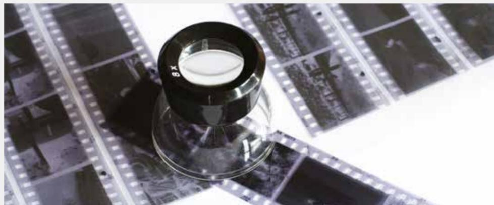
FIGURE 2 A developed film roll: the darkened areas represent where the silver has precipitated.
