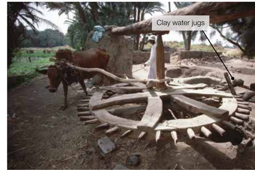
Source 3 Wooden waterwheels were another important irrigation technology in ancient Egypt. This traditional waterwheel near Luxor, Egypt, is similar in design to those used in ancient times. The water comes out of the well on a second wheel carrying clay water jugs (shown to the right). This water then supplies the irrigation network.
