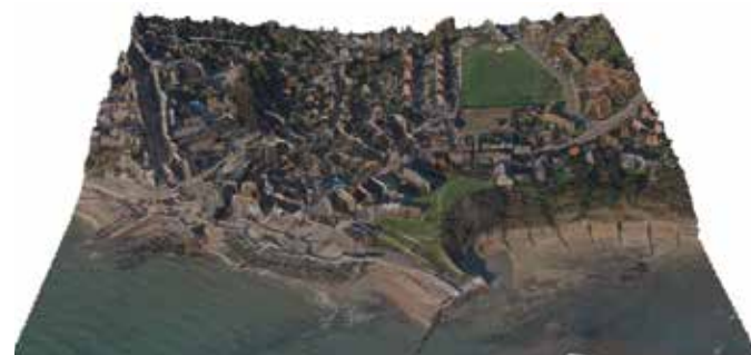
Source 3 The same data used to create the first DTM has been combined with an aerial photograph to create a more realistic digital representation of the landscape.
