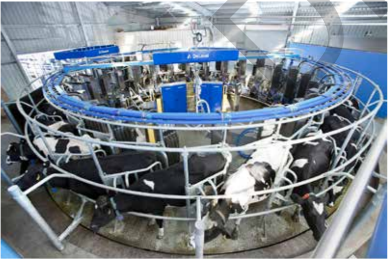
Source 4 Automation being used to milk cows in what is called FutureDairy. The cows enter the 16 milking points and a robotic arm washes the teats and attaches a cup so that milk can be extracted.
