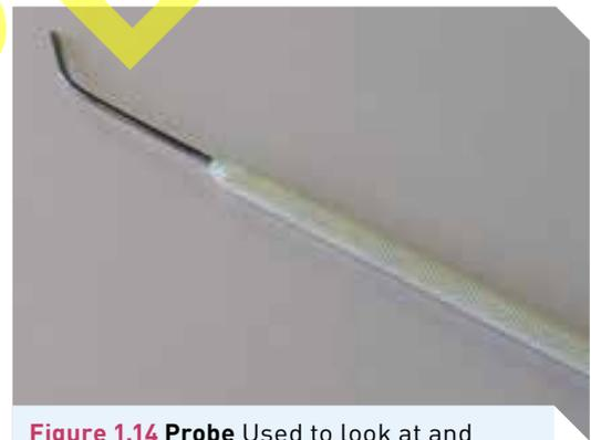
**Figure 1.14 Probe** Used to look at and explore a specimen, and to probe openings.
