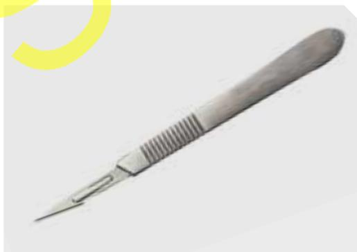
**Figure 1.15 Scalpel** Small and extremely sharp steel blade used for precision cutting.
