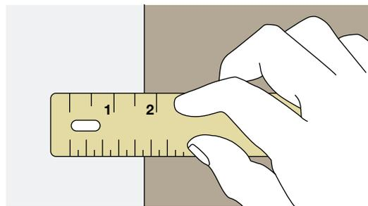
**Figure 1.5** Guessing the measurement between units of measurement (for example, between 1.5 and 2) can produce a reading error.
