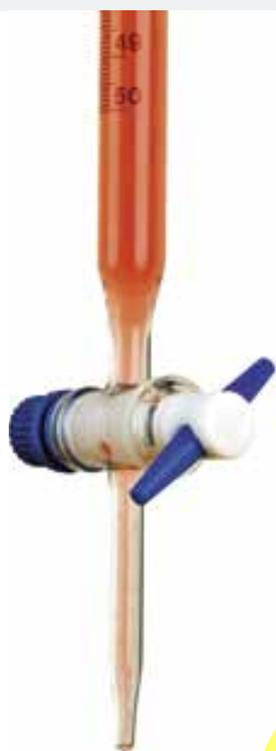
**Figure 1.4** A burette is a laboratory instrument used to accurately measure the volumes of liquids.
