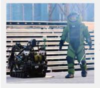
Source 3 Robots are now used in many fields and industries such as medicine, manufacturing, the military and the police. This robot is being used by the Civil Defence Force in Singapore to defuse and dispose of a bomb during a training drill.
