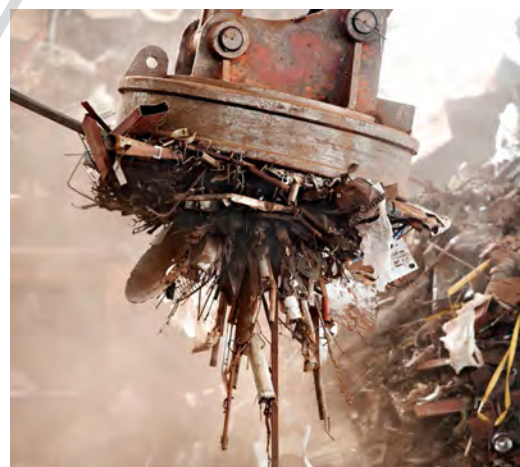
Figure 3.12 Magnets are used to separate metals in recycling plants.
