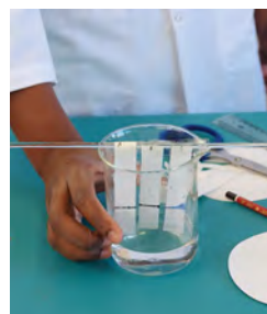
Figure 10.35 Hang the paper strips over a glass rod so they just dip into the salt solution.
